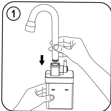
**GB** Insert the faucet piece into the pump until you hear a locking sound, the faucet piece cannot be taken out again.
