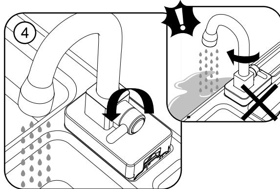
**(GB)** Turn on the pump to activate water flow. The faucet turns at 360 degree, please make sure that the faucet faces toward the sink to avoid water flow unexpectedly.
