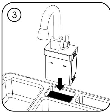
**(GB)** Insert the faucet and pump into the open hole of the sink cover, push in until you hear a locking sound.
