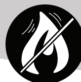
NOISY FLAME (EXCESSIVE OXYGEN)
