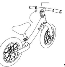
Hold handlebar in correct position and tighten the 2 screws. Re-tighten the top cap.
