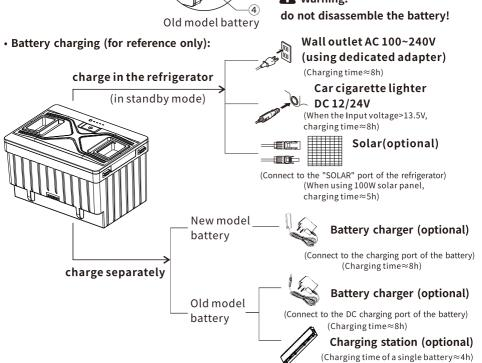
**Note:** It is suggested to switch off the refrigerator when charging the battery (the power supply may mainly power the compressor when the refrigerator is running).
