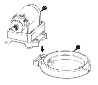
5. Insert and push the Lock Pins <sup>1</sup> all the way down to secure the Pump <sup>1</sup> to the Sand Tank Base <sup>1</sup>.
