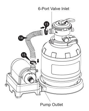
18. The sand filter pump is now fully assembled. To install it to the pool, connect the Pump Inlet to the pool Outlet with a Long Hose and one Clamp on each end. Then connect the 6-Port Valve Outlet to the pool Inlet with another Long Hose and Clamps. Tighten all the Clamps with a flat-blade screwdriver.
