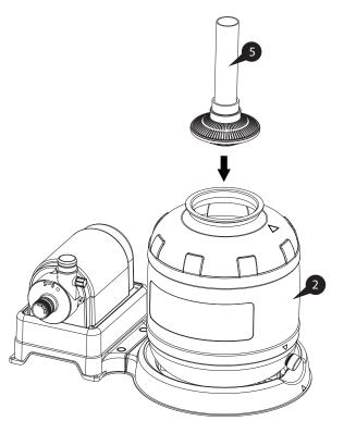
8. Place the Sand Guard **6** over the top opening of the Center Pipe **6**.
