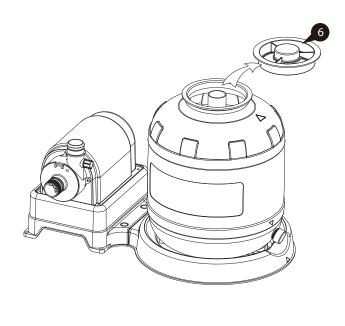
11. Install the 6-Port Valve to the Sand Tank 2, and ensure if fits securely into the Center Pipe 5.
