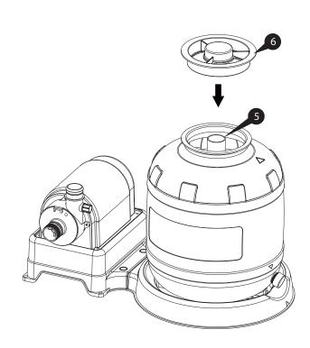
9. Fill the tank with #20 silica sand ONLY.
