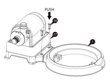
With the Drain Valve of the Sand Tank pointing outwards, place the Sand Tank onto the Sand Tank Base .
