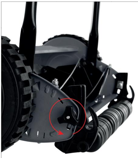
Lift the mower up onto a workbench, and insert a piece of paper in between the blades and the cutting edge (B).
