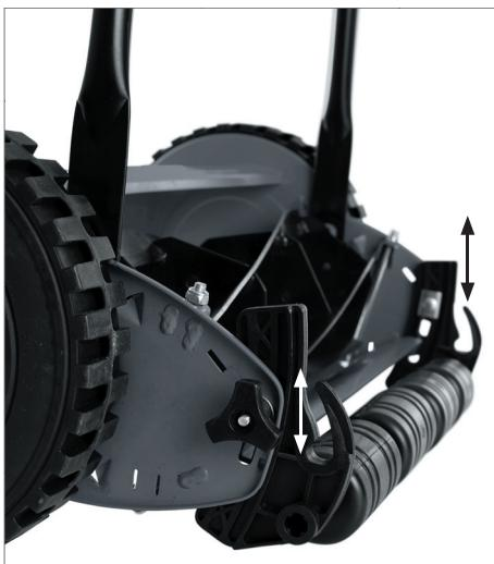
Check regularly that the cutting mechanism is set correctly.
