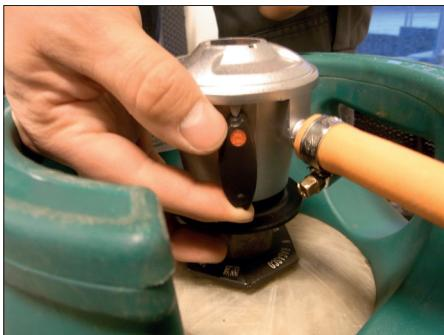
Press the adjustment button and turn it anticlockwise to the dot after the "PILOT" position (see the arrow in the illustration).
