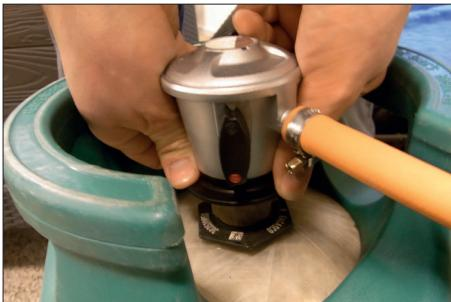
The regulator must be tight so that it is possible to lift the gas bottle just by holding on to the regulator.
