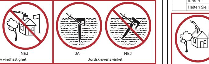
JORDSKRUVARNA SKA TRYCKAS RAKT NER TILLS DEN ÖVRE ÄNDEN BEFINNER SIG UNDER MAR-KNIVÄ. TRYCK INTE I JORDSKRUVARNA SNETT.
